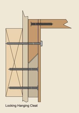
Anchorage fasteners are required to achieve a minimum penetration of 38.1mm [1.500"] into the wall studs, in-wall blocking, or masonry walls.
