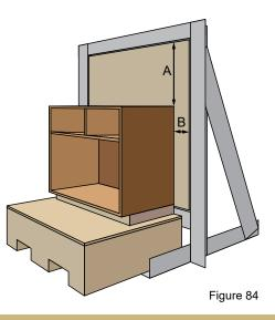
Install test specimen plumb and level within 1.6 mm [.063"] over 2.44 meters [8'] in both vertical and horizontal axis.
